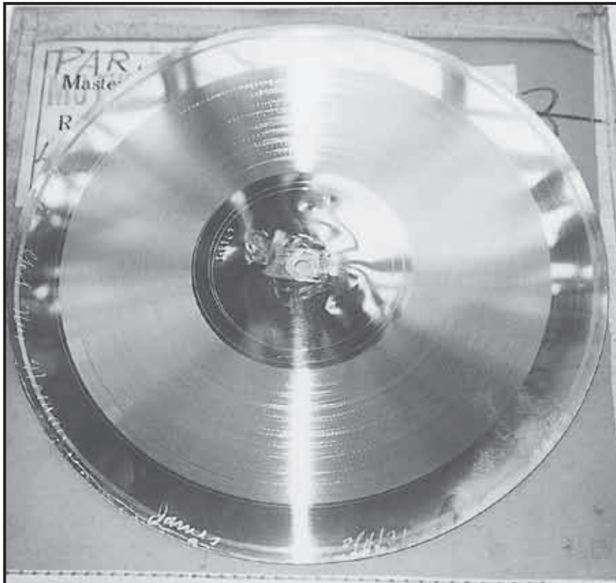
This metal mother of Skip James' 'Devil Got My Woman' (mx. L-746) is one of the few surviving NYRL metal parts. From 'Paramount's Rise and Fall'. Courtesy Alex van der Tuuk
